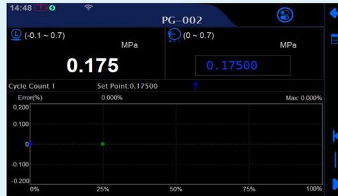
Pressure gauge / transmitter / switch calibration
