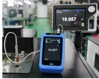
Additel's 282 Reference Thermometer Readout utilizes a ratio measurement technology which provides an unmatched performance in stability and drift. In order to ensure a very small temperature drift coefficient and reliable long-term stability, the ADT282 uses current reversal techniques to cancel EMF effects and a ratio technology to cancel the A/D converter offset. This highly advanced technology has not been available in a handheld device until now!
